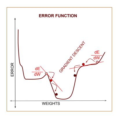
error = (desired target - actual output) new\_W =  $(old_W - Ir * \frac{dE}{d(old_W)})$
