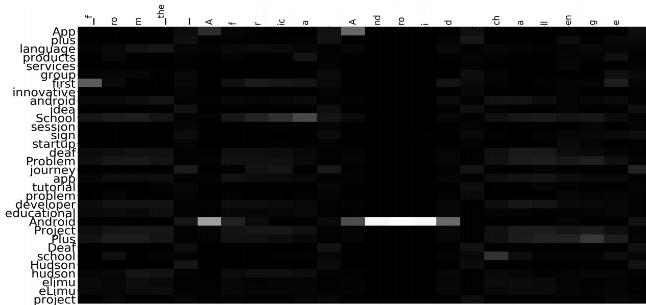
Figure 3: Visualizing attention weights, \alpha_{u,n} from Equation (5c), for the example in Table 1, row 1. The x-axis shows the target units from the hypothesis output by the Contextual RNN-T Model, and the y-axis shows the contextual metadata words ( w_i ). Darker colors represent values close to zero while brighter colors represent values closer to 1.
