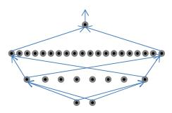
A network with less than 16 neurons in the first layer cannot represent this pattern exactly ...
