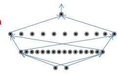
A 2-layer network with 16 neurons in the first layer cannot represent the pattern with less than 40 neurons in the second layer
