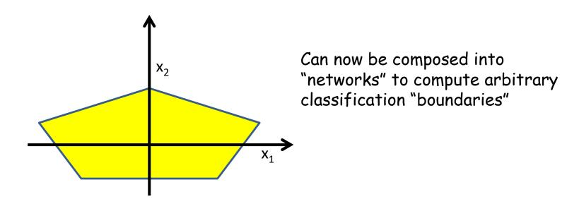
Build a network of units with a single output that fires if the input is in the coloured area
