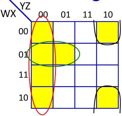
$$O = \bar{Y}\bar{Z} + \bar{W}X\bar{Y} + \bar{X}Y\bar{Z}$$
