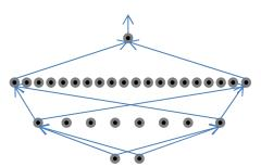
A network with less than 16 neurons in the first layer cannot represent this pattern exactly
