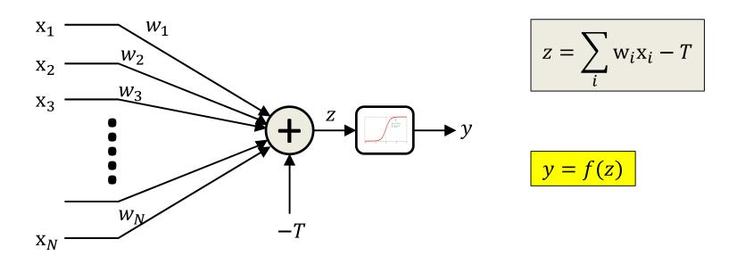
The output of the neuron is a function of a linear combination of the inputs and a bias
