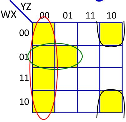
$$O = \bar{Y}\bar{Z} + \bar{W}X\bar{Y} + \bar{X}Y\bar{Z}$$
