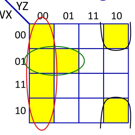
$$O = \bar{Y}\bar{Z} + \bar{W}X\bar{Y} + \bar{X}Y\bar{Z}$$
