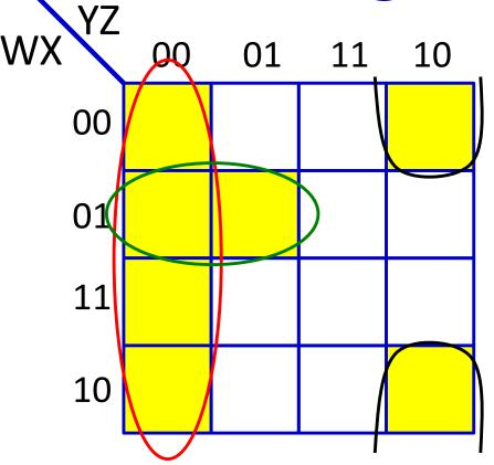
$$O = \bar{Y}\bar{Z} + \bar{W}X\bar{Y} + \bar{X}Y\bar{Z}$$
