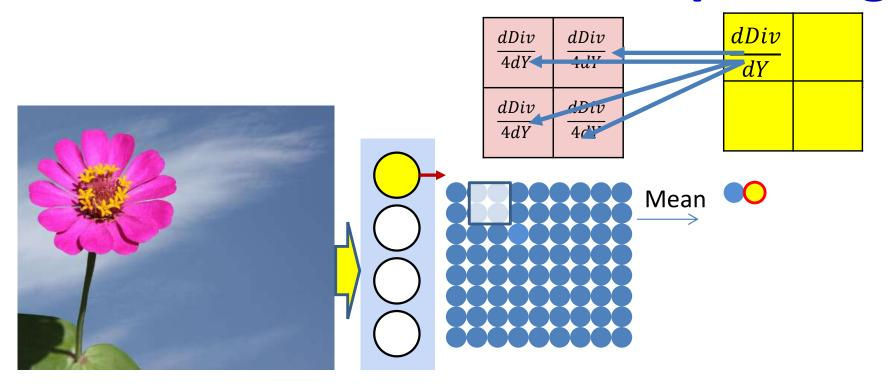
The derivative of mean pooling is distributed over the pool
