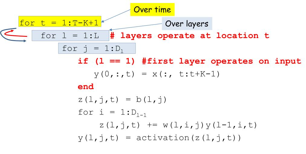
Scanning with an MLP Over layers for 1 = 1:L # layers operate at location t for t = 1:T-K+1  $\longleftarrow$  Over time for  $j = 1:D_1$ if (1 == 1) #first layer operates on input y(0,:,t) = x(:, t:t+K-1)end z(l,j,t) = b(l,j)for  $i = 1:D_{1-1}$ z(l,j,t) += w(l,i,j)y(l-1,i,t)y(l,j,t) = activation(z(l,j,t))
