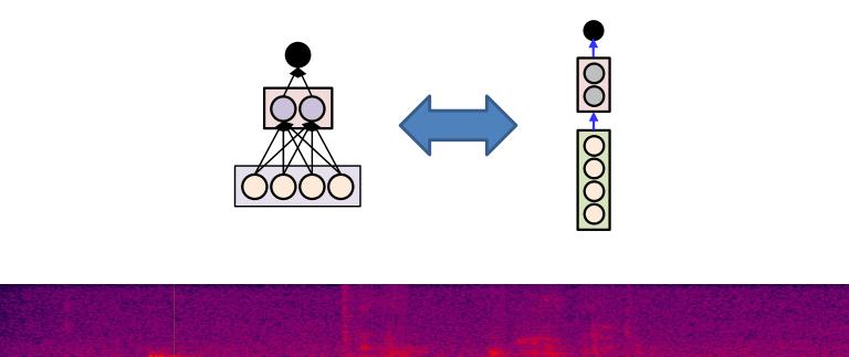
The 1-D scan version of the convolutional neural network is the *time-delay neural network* Used primarily for speech recognition
