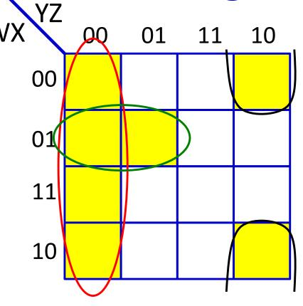
$$O = \bar{Y}\bar{Z} + \bar{W}X\bar{Y} + \bar{X}Y\bar{Z}$$
