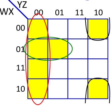
$$O = \bar{Y}\bar{Z} + \bar{W}X\bar{Y} + \bar{X}Y\bar{Z}$$
