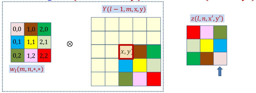
$$z(l, n, x', y') += Y(l-1, m, x, y)w_l(m, n, x - x', y - y')$$
