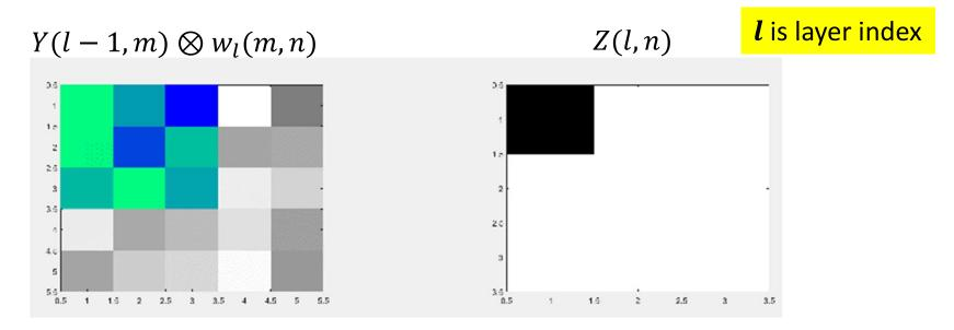
$$z(l, n, x, y) = \sum_{m} \sum_{x', y'} w_l(m, n, x', y') y(l - 1, m, x + x', y + y') + b_l(n)$$
