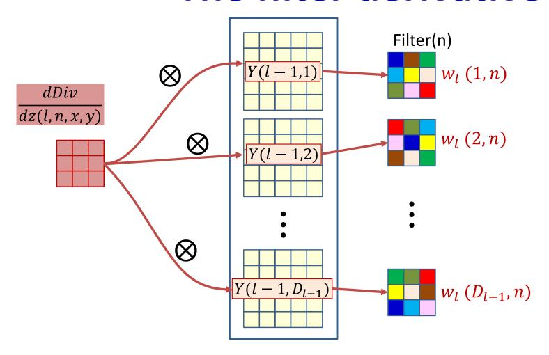
• The derivative of the  $n^{th}$  affine map Z(l,n) convolves with every output map Y(l-1,m) of the (l-1)<sup>th</sup> layer, to get the derivative for  $w_l(m,n)$ , the  $m^{th}$  "channel" of the  $n^{th}$  filter
