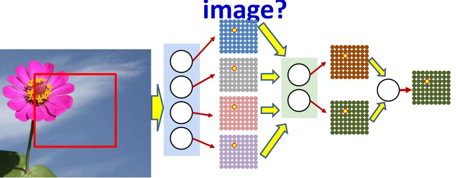
To detect a picture at any location in the original image, only need to consider the corresponding location of the output map
