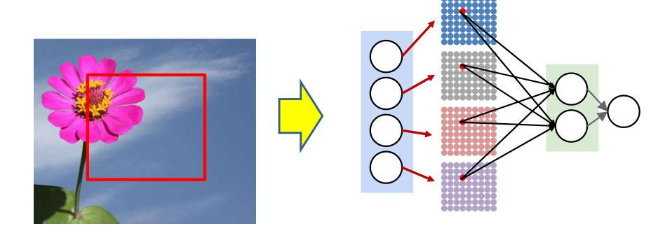
To classify a specific "window" in the image, we send the first level activations from the positions corresponding to that position to the next layer
