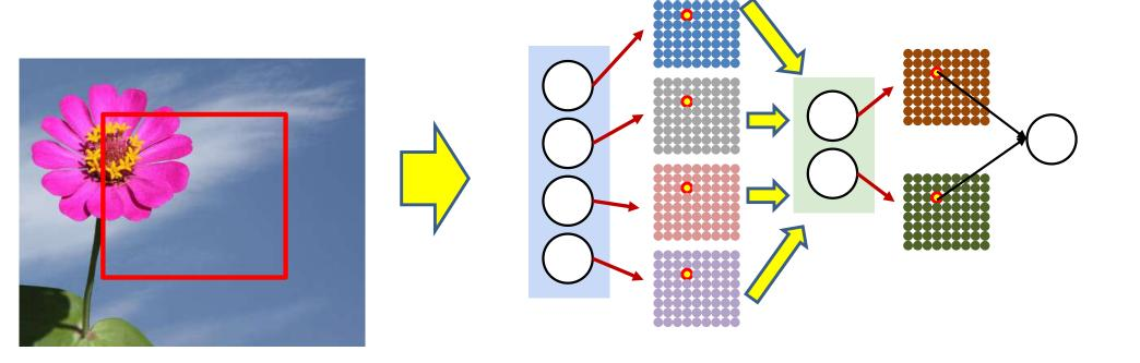
To detect a picture at any location in the original image, the output layer must consider the corresponding outputs of the last hidden layer
