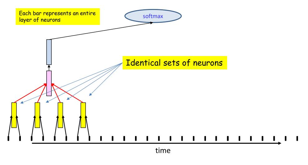
Scan of 8-time-step wide patterns with a stride of two time steps distributed over two layers
