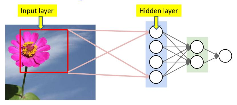
The "input layer" is just the pixels in the image connecting to the hidden layer
